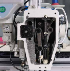
机头无油 Oil-free in the machine head
