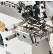
周长148mm小缝台设计 Small sewing table design with a circumference of 148mm
